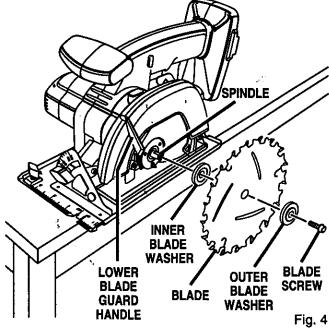
Note: Turn blade screw clockwise to remove.
